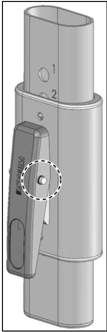
Diagram 13: If needed, lubricate the pivot pin on the ratcheting seat lever
